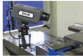
FLIR thermal imaging camera for heat evaluation
