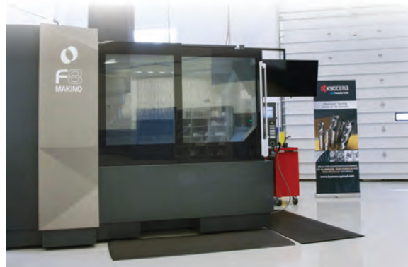
Incorporation of innovative machine tool technology for Research and Development including the Haas VF3SS-30/VM3-30 (15,000 rpm) and Makino F8-50 (10,000 rpm)
